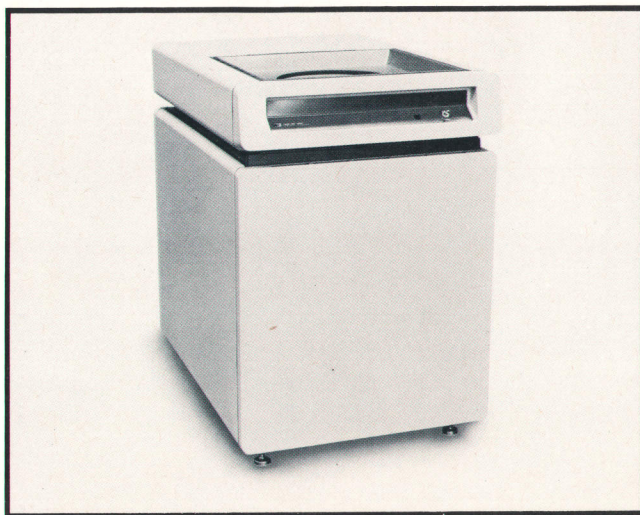
Fig. 1. Model 7920A Disc Drive provides a 50M-byte formatted storage capacity for HP 1000, 2000, and 3000 Computer Systems. Average access time is 25 milliseconds. Up to eight drives can be interfaced to one disc controller.
